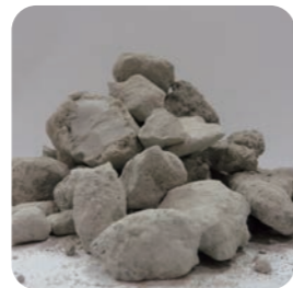
Recycled roadbed material
