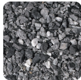
Crushed sand for concrete
