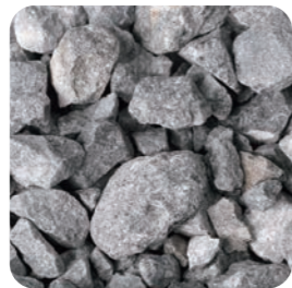
Crushed stone for concrete
