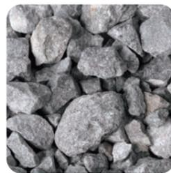
Crushed stone for concrete
