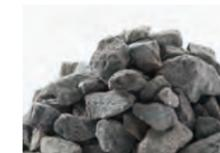
Crushed stone for concrete
