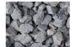
Crushed stone for concrete
