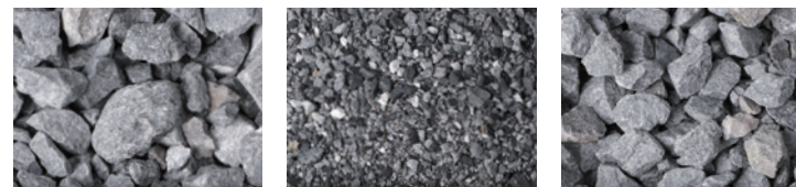
Crushed stone for concrete Crushed sand for concrete Crushed stone for roads
